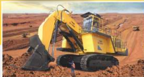
BE1800 EI. Excavator (Operating Wt. 180 Ton)
