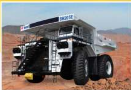
BH205E DUMP TRUCK (Pay load 190-205 Ton)
